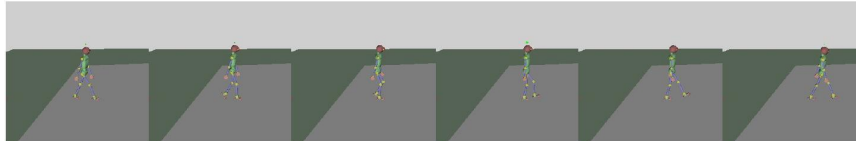
Fig. 2. A part of the stride of the simulated biped walking on the 5° upslope
