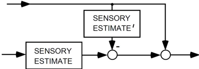
**Figure 2 Principle of fusing sensory estimates of external disturbance with predicted-sensory disturbance estimates.**
